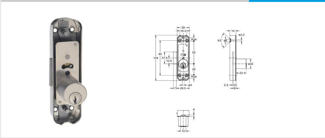
The technical drawings show a front view of the lock with dimensions: 104mm height, 28mm width, 16.2mm top offset, 80mm distance to center, 27.6mm to internal feature, 13.5mm to bottom, 52mm to internal feature, 25mm to bottom, 17mm to side, 29.5mm to bottom, and 4mm to side. A side view shows a 90-degree angle, 14mm offset, 3.2mm diameter hole, 23mm distance to bottom, and 2.3mm and 6mm dimensions at the base. A detail view shows a 4mm high feature on a 12mm wide base.
